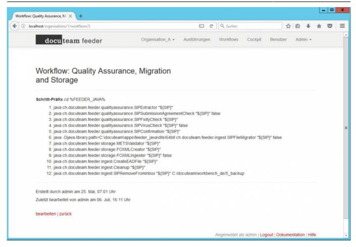
The link "edit" und "Bearbeiten" leads to a page in which workflows can be edited. A workflow always has a linear progression: Basically, a SIP is sent into a pipeline, in which each step is processed successively. In case of an error, the process is stopped and the pending steps are omitted.
